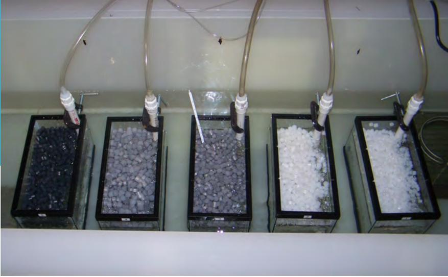
Side-by-side testing validates performance at 800 m<sup>2</sup>/m<sup>3</sup> surface area.
