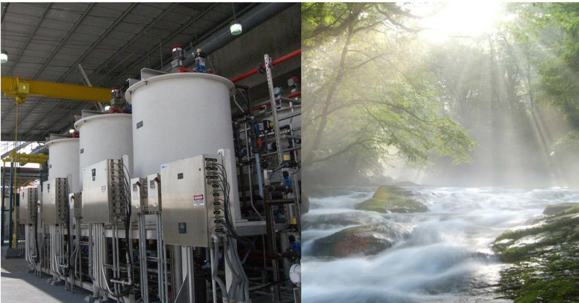
The EcoRegen® System is an ultra low-waste ion exchange regeneration system that further reduces the ecological footprint of the MIEX® Process.
