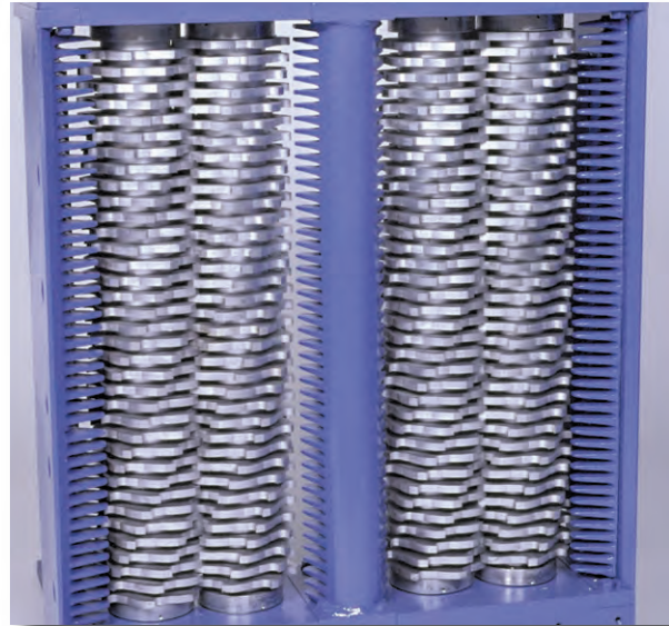
A unique, pressure-balanced center post allows the flow to pass freely and optimizes performance.
