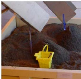
Sandbox grade grit is produced by the RoSF4 Coanda® system while it funnels the organics into a treatment process. The end-result is two useful – not harmful – by-products. The grit – once offensive and hazardous – is now a popular cover material used at the City’s landfill.
