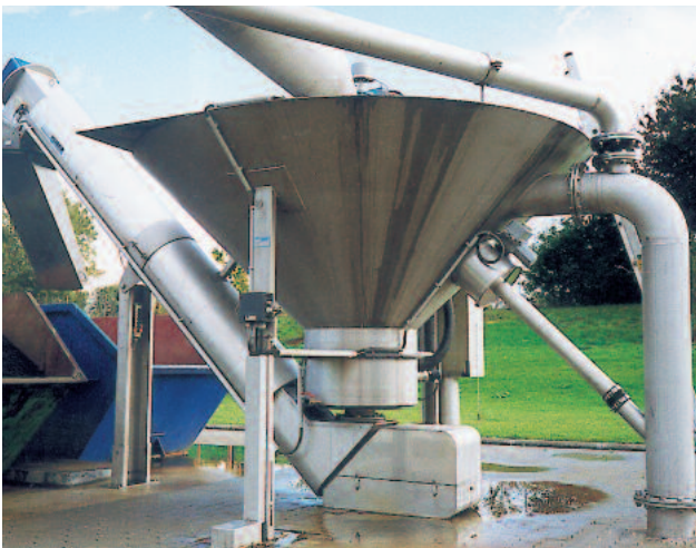
COANDA Grit Washer RoSF 4 / Size III with frost-protection for outdoor installation
