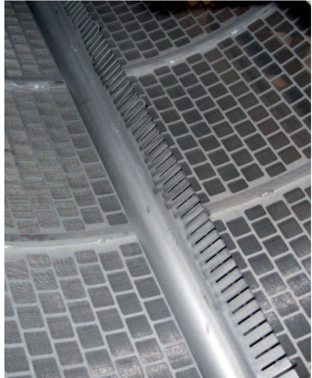
View of the internal drum. A center feed drum design provides the best solution for protection of MBR.
