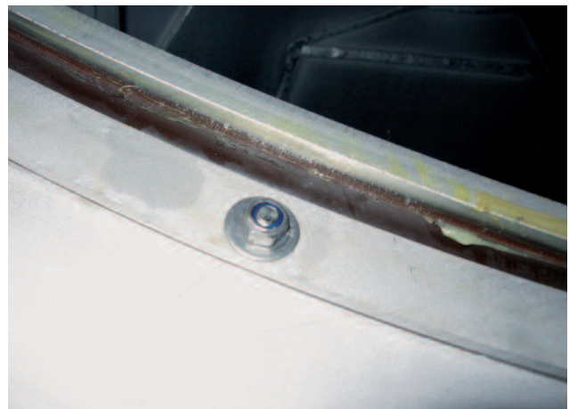
The RoMem utilizes a polyurethane drum seal. This is critical for proper sealing to assure bypass protection.
