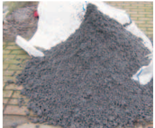
Screenings discharged from a HUBER Wash Press WAP
