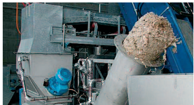
Well washed and virtually odorless screenings from a WAP/SL, compacted to 50 % DS
