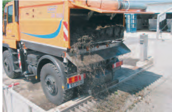
Acceptance tank with bar grate and integrated horizontal dosing screw
