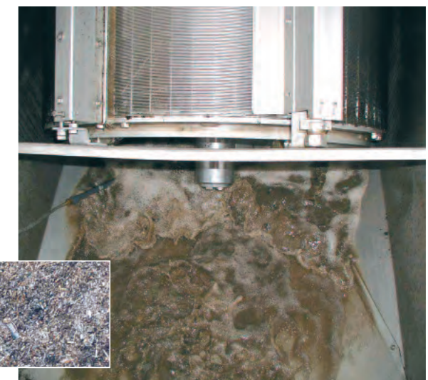
ROTAMAT® fine screen for 1 mm screening and dewatering of organic material (approx. 30 % DR)
