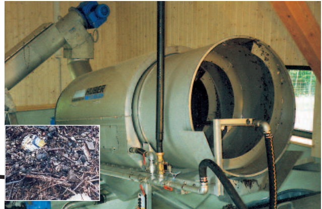
ROTAMAT® Wash Drum for washout and separation of all coarse material > 10 mm
