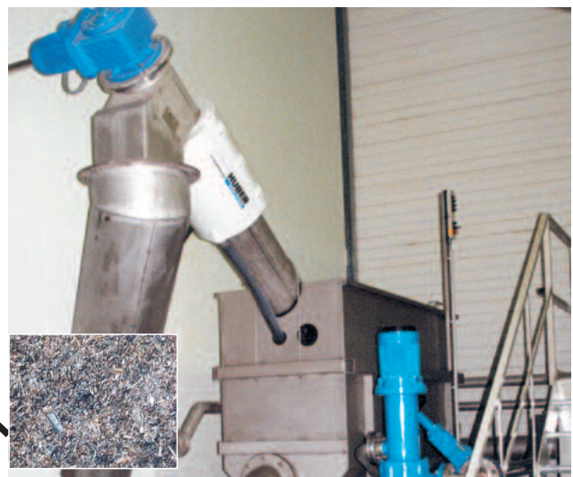
ROTAMAT® fine screen for 1 mm screening and dewatering of organic material (approx. 30% DR)
