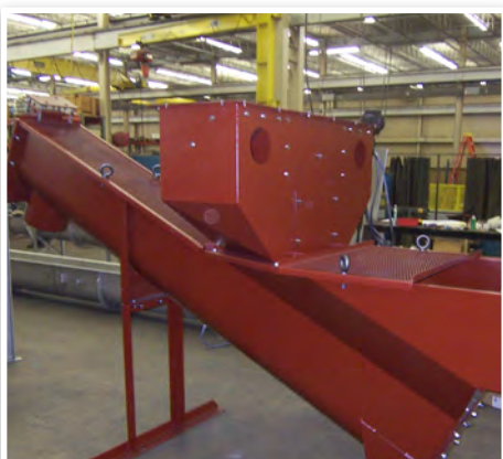
Shafted classifiers can be equipped with a screw lift assembly for ease of maintenance.
