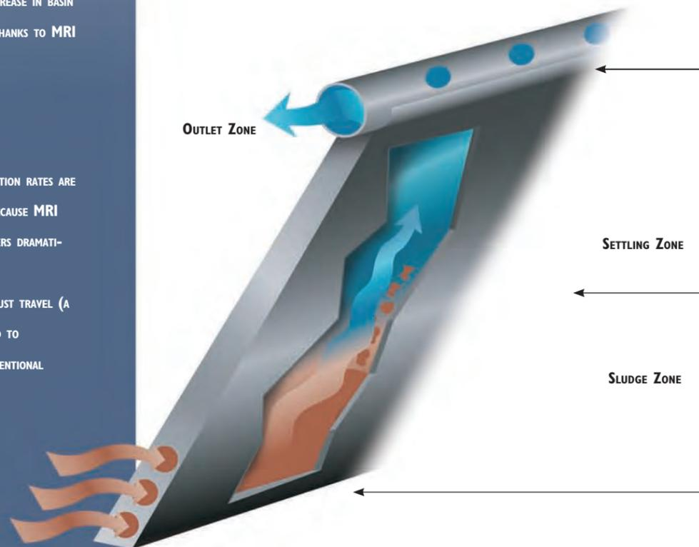
AS CLARIFIED WATER IS DISCHARGED FROM THE EFFLUENT TUBES AT THE TOP OF THE PLATES INTO THE EFFLUENT TROUGHS, MRI'S MICRO-ADJUSTABLE WEIR ALLOWS FOR PRECISE CONTROL OF FLOW VELOCITY AND EQUALIZATION FOR ENHANCED EFFICIENCY.
