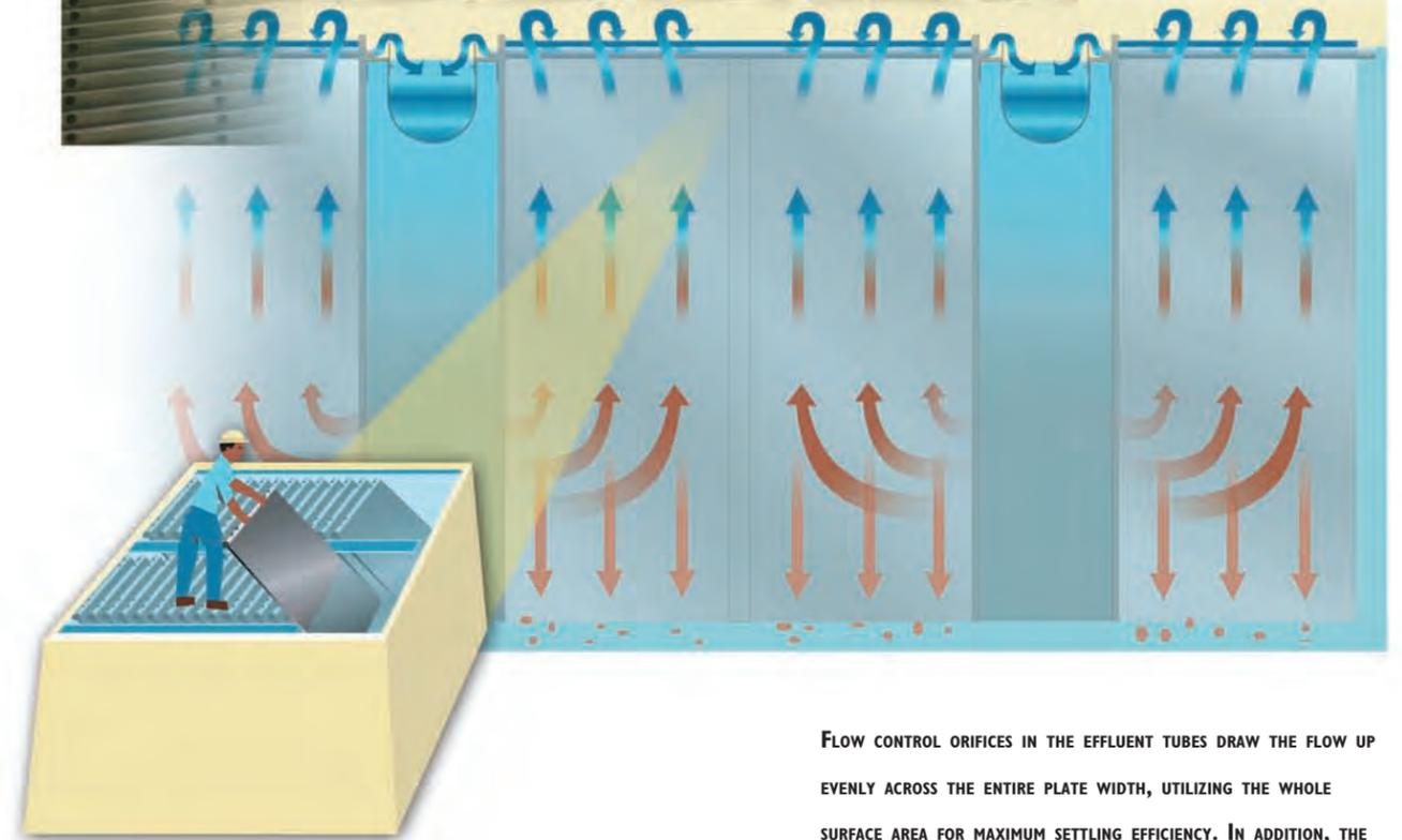
**FLOW CONTROL ORIFICES IN THE EFFLUENT TUBES DRAW THE FLOW UP EVENLY ACROSS THE ENTIRE PLATE WIDTH, UTILIZING THE WHOLE SURFACE AREA FOR MAXIMUM SETTLING EFFICIENCY. IN ADDITION, THE INFLUENT FLOW IS INTRODUCED ACROSS THE PLATE FROM THE LOWER SIDE, RATHER THAN STRAIGHT UP FROM THE BOTTOM, ENSURING MINIMUM INTERFERENCE WITH DOWN-FLOWING SLUDGE.**
