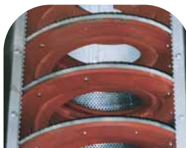
Heavy-duty spiral conveys the screenings to a dewatering zone
