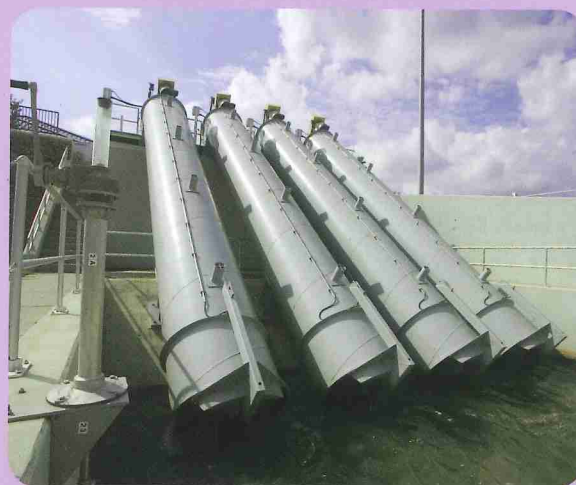
Tube Mounted Screw Pumps with a stationary outer shell eliminate the need for a precisely grouted concrete channel. Available with fixed or variable angle of inclination for control of pumping rates. Sizes from 20" to 72" in diameter. Lift capability up to 25'.
