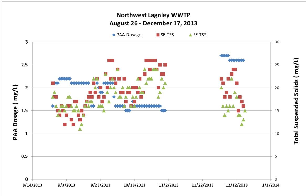
**Figure 5: Comparison of total suspended solids of the final effluent and secondary clarifiers at various PAA doses**
