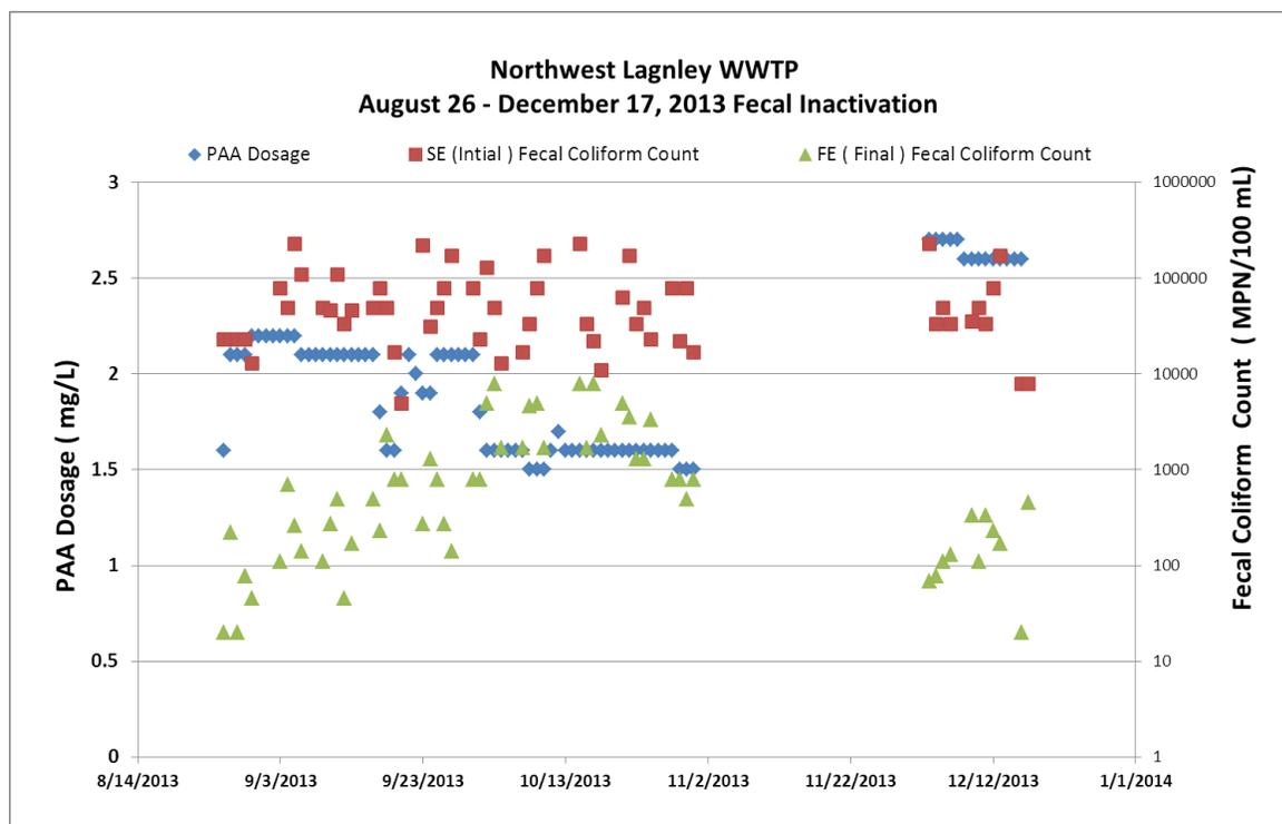
**Figure 4: NWLWWTP fecal coliform inactivation using PAA as disinfectant between August 26<sup>th</sup> and December 17<sup>th</sup> 2013**
