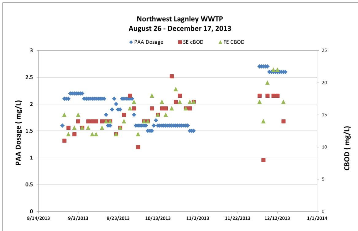
**Figure 6: Comparison of cBOD of the final effluent and secondary effluent at various PAA doses.**
