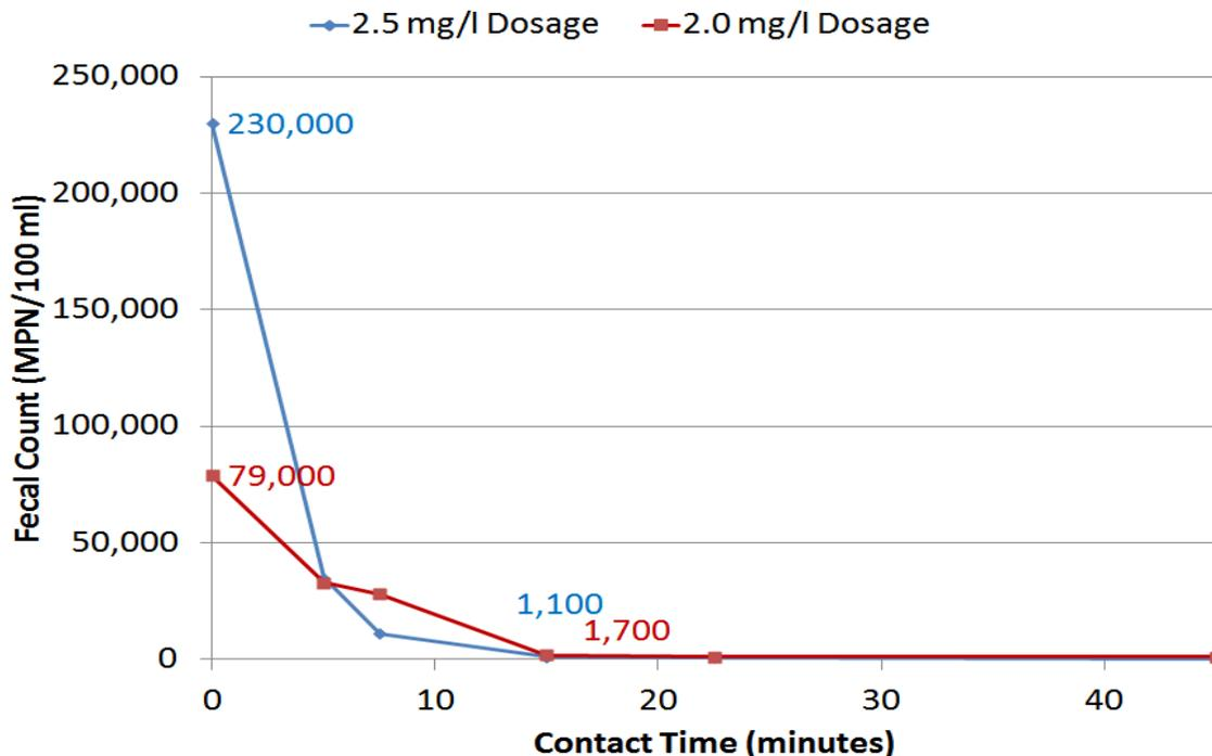
**Figure 7: Fecal coliform inactivation kinetics**
